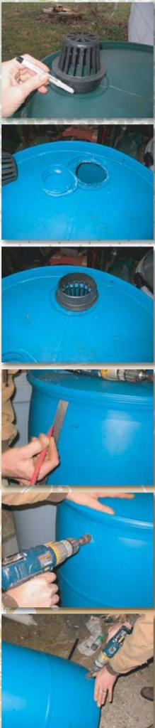
Drill hole using 1" holesaw from bottom of the barrel.
